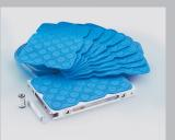
VAC-MAT is vacuum chuck that comes covered with elastic plastic mats. The thin, soft mats are provided with vacuum suction holes, through which the air between workpiece and mounting surface is sucked out.
