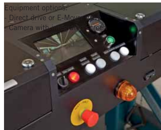
Control panel with camera monitor
