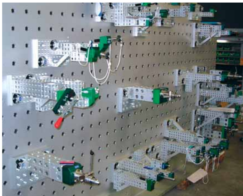
Sandwich plate mounted with PWS base plates using clutch bolts for grid 100mm
