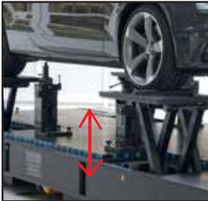
With integrated jack lift and air-cushioned and floating support plate
