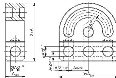
**Swivel plate with slot**swivel range  $\pm 90^\circ$ , pivot point independent of grid
