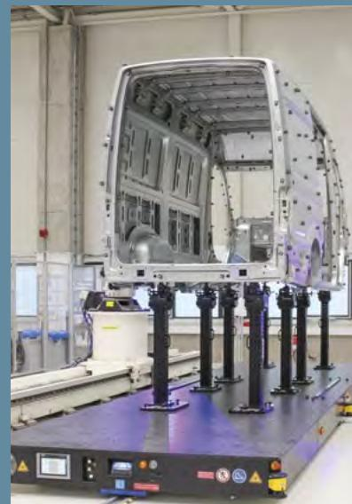
Structure plates from the Witte FixBase® range are ideally suited as a base for column type fixture design.
