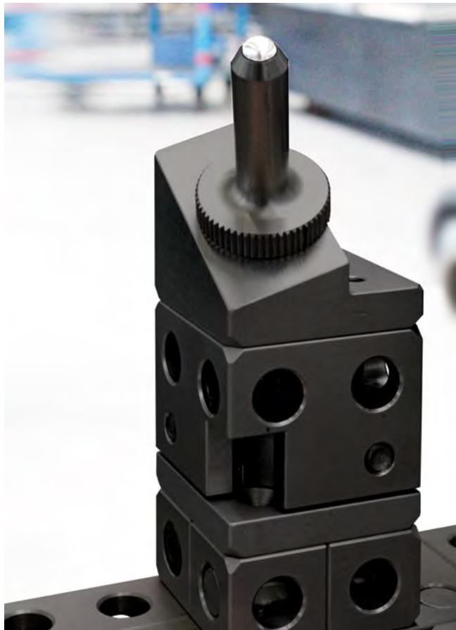
The angle of the center point is guaranteed by a specially machined contour block. The position in x, y and z is defined by the shimblock, the upper part of which is adjusted with shims in steps of 0.05 mm. Finally, the Shimblock is locked in order to achieve a permanent and stable position.
