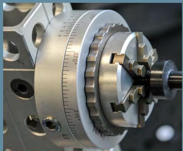
The rotary plate enables defined rotation of the elements attached to it - accurate and reproducible thanks to locking screws and scales with verniers.
