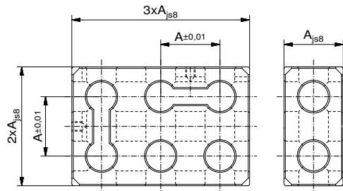
**Base plate 2D for screw connectors**
