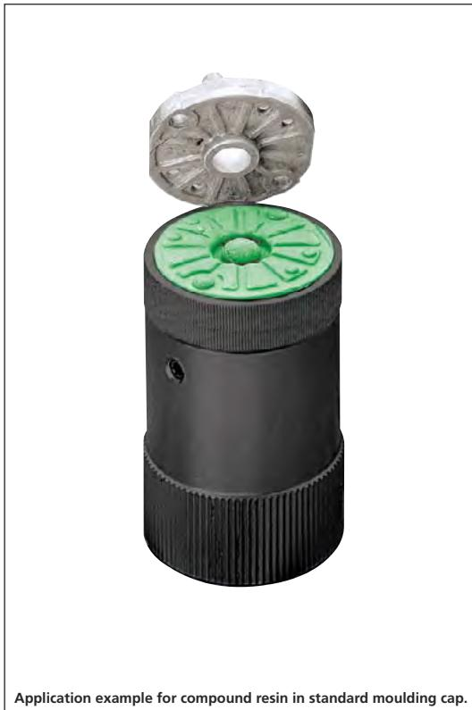
Application example for compound resin in standard moulding cap.
