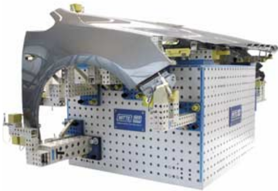
Fixbase Cube for mounting single parts of vehicle front
