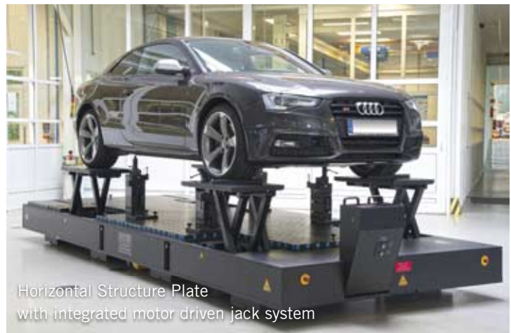
FixBase cube combination mounted with column type supports
