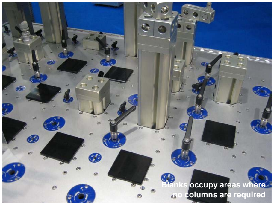
Power assisted columns set to height
