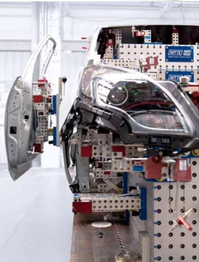
FixBase cube combination mounted with column type supports
