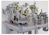
Gap and flush gauges - with folding/removable contour stripe models and or measuring equipment
