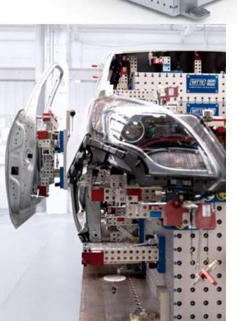
FixBase cube combination mounted with column type supports
