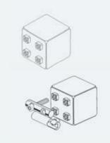
Nubs are space saving connection solution for slides, quick couplings and contour blocks.
