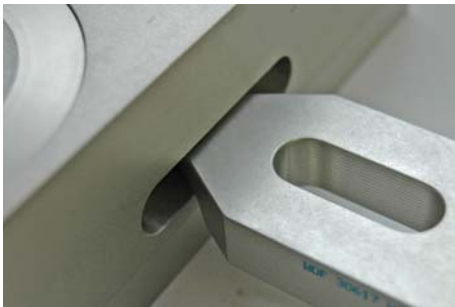
Fig. 3: Attaching the clamping jaws
