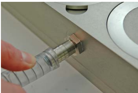
Fig. 4: Connect the vacuum hose
