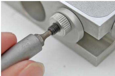
Fig. 8: Install the set screw
