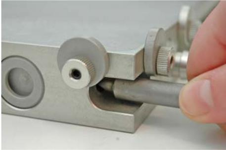
Fig. 4: Release the screws
