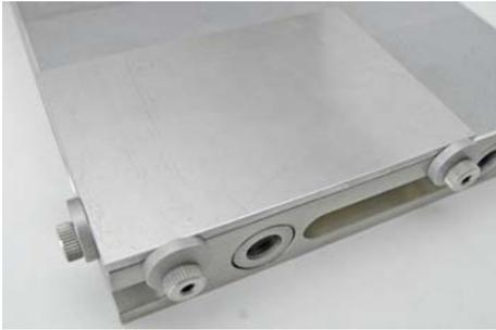
Fig. 10: Clamping the workpiece
