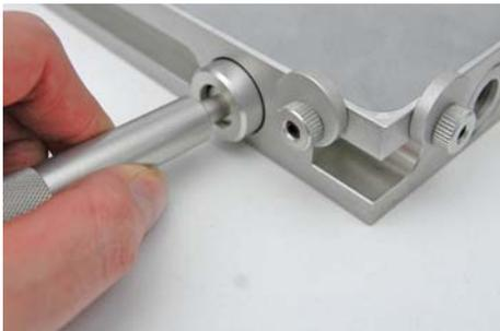
Fig. 5: Remove the blanking plugs
