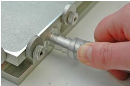
Fig. 3: Connect the vacuum hose
