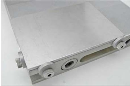
Fig. 10: Clamping the workpiece
