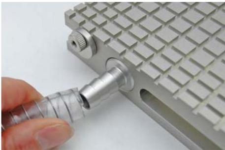
Fig. 3: Connect the vacuum hose
