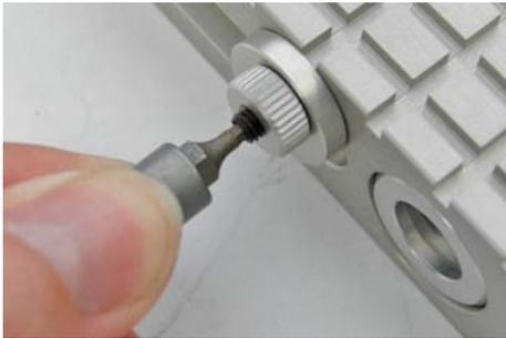
Fig. 8: Install the set screw
