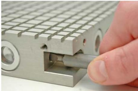
*Fig. 4: Release the screws*
