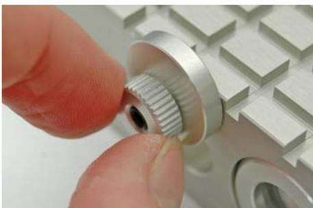
Fig. 9: Tighten the stop washer
