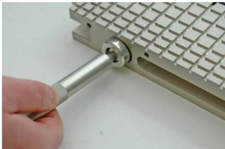
*Fig. 5: Remove the blanking plugs*
